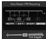
Figure S7.1 The FM algorithm selector in Surge. In this instance, the parallel modulator option has been selected.
