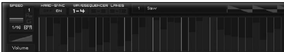
Figure 5.4 Using Wusikstation's controller lane to create gating effects.
